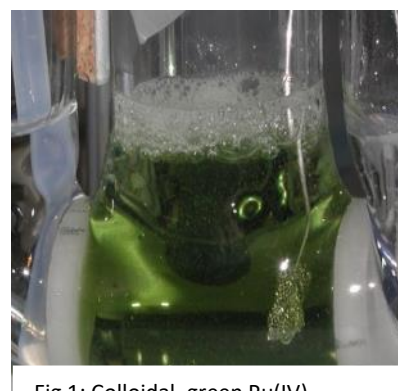
Fig 1: Colloidal, green Pu(IV) solution prepared by electrolysis.
