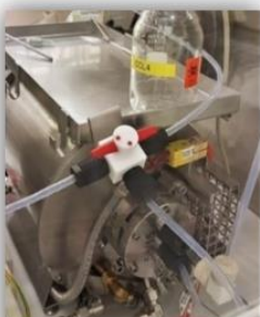
Figure 1: Chlorination furnace, inlet of gas on the left, outlet on the right
