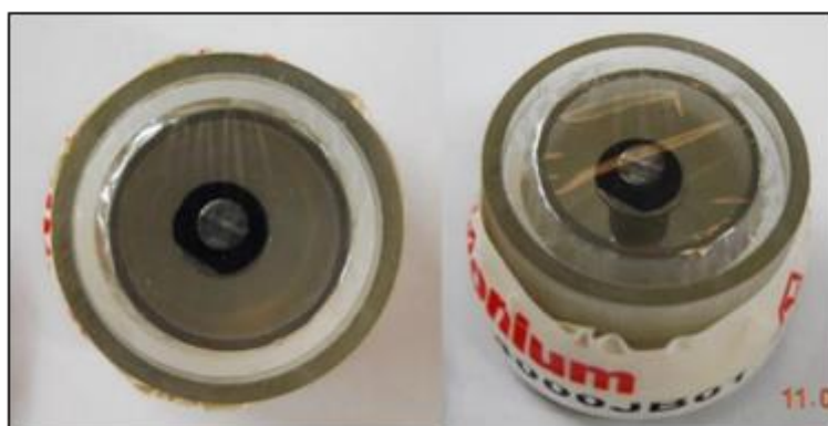
Figure 1: Example sample containment system for direct plutonium analysis in the open laboratory [1]
