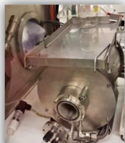
Figure 1: Chlorination furnace, inlet of gas on the left, outlet on the right
